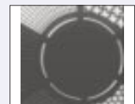
Image of a collimator using a 1.5 mm thick Silicon detector. Smallest holes are 0.15 mm dia.
