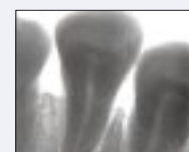
Image of a jaw with teeth using a 1.5 mm thick Silicon detector.
