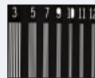
Image of a bar pattern X-ray image using a 1 mm thick Silicon detector hybrid. Nyquist limit is 10 lp/mm.
