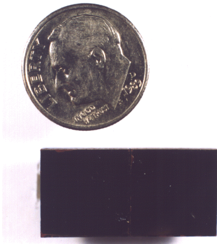
Figure 3. A position sensitive CdZnTe pad detector with 32 ( 4 \times 8 ) pads used for testing the prototype RENA chip.
